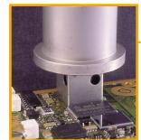
The systems are fitted with an under-board heater. The CSP version has a 1000W convection heater suitable for smaller PCBs, while the BGA version is fitted with a 1400W large area heater with the capacity to work with thermally demanding multi-layer boards. This eliminates problems associated with warped boards.
